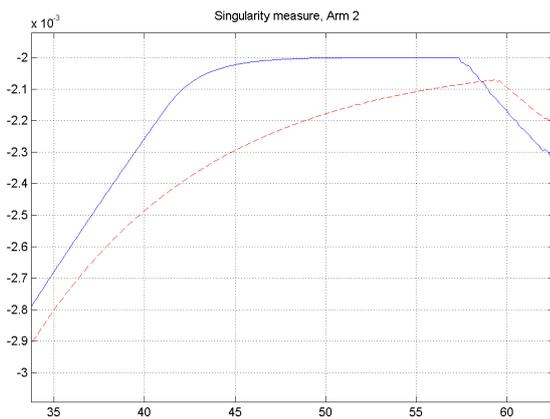
Fig. 7. Parts of the middle plot of Figure 6. Note how the bound  $b_2 = -0.002$  is approached exponentially in a worst case scenario where this produces the best decrease in  $f_1$ . Then, slightly after  $t = 57$  the, optimization produces a rapid improvement in the singularity measure. Note also how a smaller  $k = 0.1$  produces a softer convergens (red dashed) than the larger  $k = 0.5$  (blue solid).
