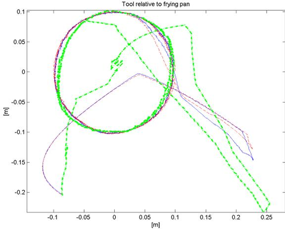
Fig. 3. The motion of the cleaning utensil in the frying pan, projected onto the frying pan plane. The results of three simulations are shown, (blue solid:  $k = 0.5, b_2 = -0.002$ ), (red dashed:  $k = 0.1, b_2 = -0.002$ ), (green dash-dotted:  $k = 0.5, b_2 = -0.005$ ).
