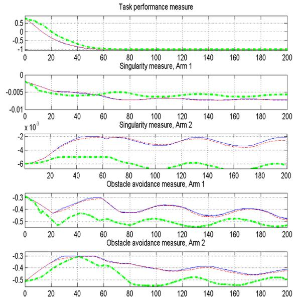
Fig. 6. Time evolution of the functions  $f_i(q)$ . Note how the scalar inequalities  $f_i \leq b_i$  are satisfied for the different settings (blue solid:  $k = 0.5, b_2 = -0.002$ ), (red dashed:  $k = 0.1, b_2 = -0.002$ ), (green dash-dotted:  $k = 0.5, b_2 = -0.005$ ).
