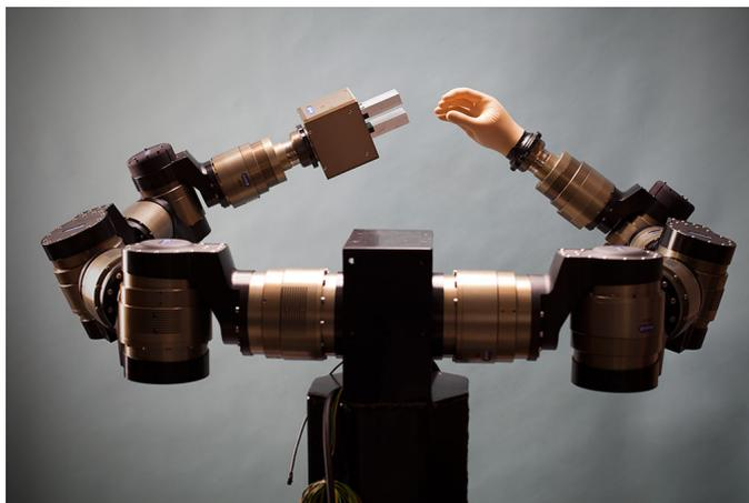
Fig. 1. Semi-anthropomorphic robot at CAS/KTH. Future work includes adapting and implementing the proposed approach to this dual arm manipulator.
