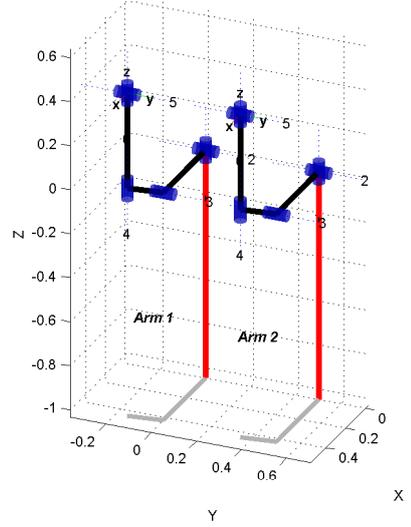
Fig. 2. The dual arm manipulator of the simulations is composed of two Puma 560 manipulators sharing the same workspace. An obstacle in form of a table is introduced at height  $z = -0.6$ .
