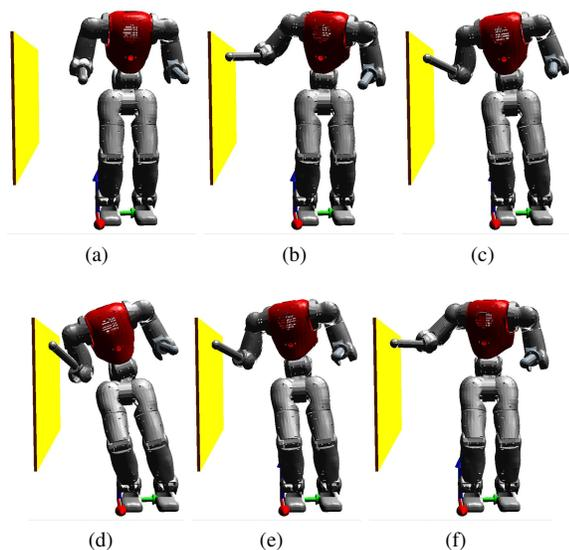
Fig. 1: Test 1: the robot made contact on the yellow wall; then it moved its COM towards the wall and back.
