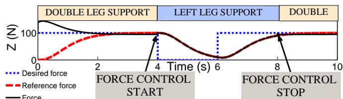
Fig. 2: Test 2: force on the right foot (normal direction).
